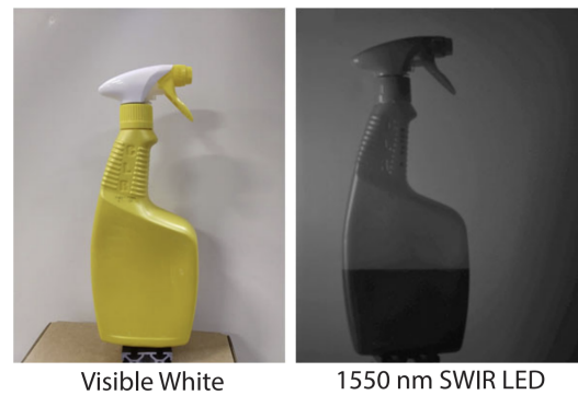
Figure 5: A 1550 nm SWIR light can enable a SWIR camera to see through a plastic container and show the fluid level.
