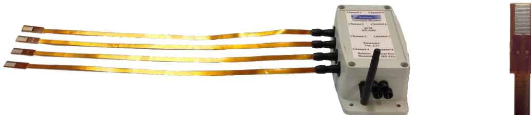
Figure 1. Wireless CHMS consisting of one AN110 node connected to four \mu LPR sensors (left) and a close-up image of a \mu LPR sensor (right).
