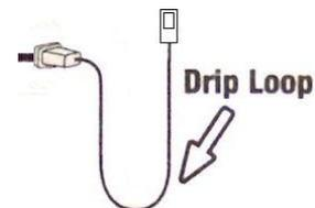
**NOTE 4:** When affixing the Relative Humidity & Temperature sensor cable to the structure, the sensor end should be oriented slightly downward to allow for proper drainage of any condensing moisture occurring inside the acrylic end tube.
